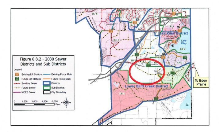
Per the Comprehensive Plan, a lift station at Powers Boulevard south of Highway 212 is required for sanitary sewer extension. The city has met with the Bluff Creek Golf Course owners and it does not appear there are any plans to develop the golf course in the near future, so development along Highway 101 is premature per the Comprehensive Plan.
